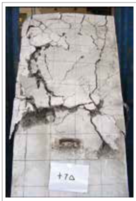
Bend bars anchor test result
